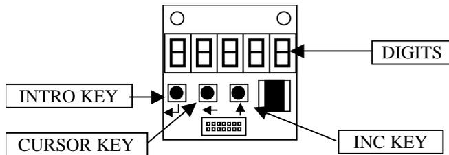
The device does not need the display board in order to work. This board is only used as an interface between the MP410 and the user. Therefore, it may be connected any time you need dialogue or to view data and disconnected afterwards without affecting the operation.
